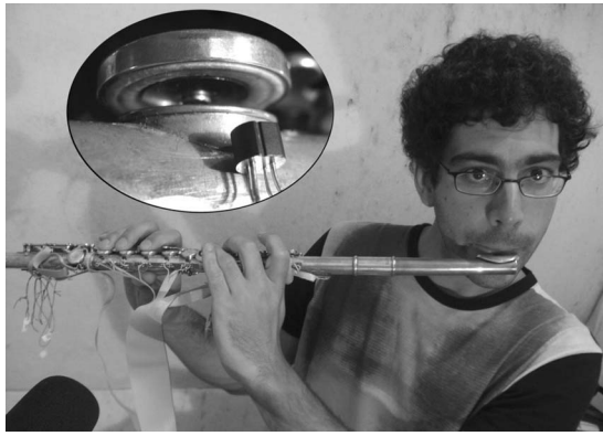
FIG. 3. An author (AA) demonstrates the modified flute used for this work. The 50 wire ribbon cable that connects the flute to the sensor electronics is visible below the flute. The microphone can be seen in the lower left corner. The inset shows how a photosensor is mounted below a key.
